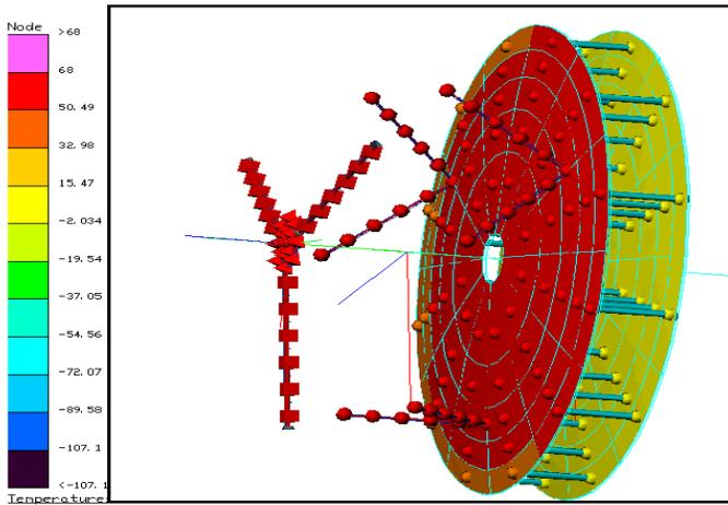
Figure 3: Thermal Desktop Model, Internal View of Detector and Primary Mirror
